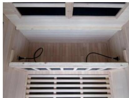
B. Slide down the bench emitter panel by lining up its sides with the vertical guides on each side panel. The emitter grid will face outward, toward the front of the sauna. Push the bench emitter panel all the way down until it is touching the floor panel and is secured in place.
