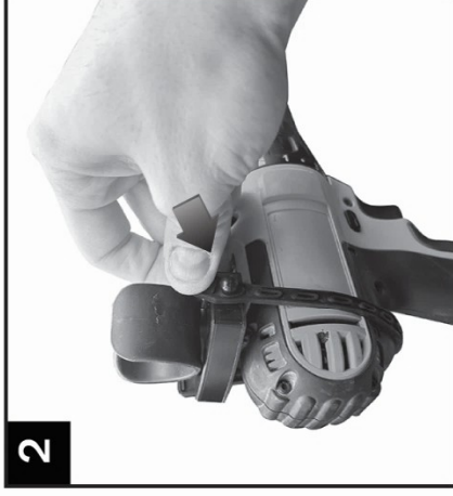
Wrap strap around tool and connect to ball socket
