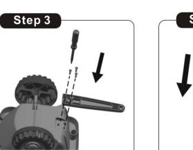
3. Assemble the trailer connector with three sliver screws by a screwdriver(not included)
