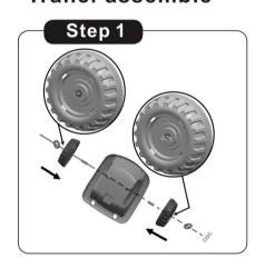
1. Insert the wheel axle through washer,trailer wheel,plastic ring into the trailer, tighten using a cotter pin.
