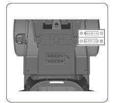
Turn over the tractor body, and find the battery house. Loosen the screw with a screwdriver(not included). Put 2 AA batteris in the battery house, then tight the screw with a screwdriver(not included).
