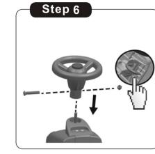
6.Loosen the bolt and nut in the steering wheel first, then place the steering wheel over the J-sharped stick, insert the bolt and tighten the nut with a screwdriver(not included)
