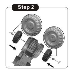
2. Insert the wheel axle through washer, rear wheel, plastic ring into the body, tighten using a cotter pin
