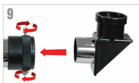
Locate the erect image diagonal and remove the plastic covers. Insert the barrel of the diagonal into the focuser and secure it in place by tightening the thumbscrews.
