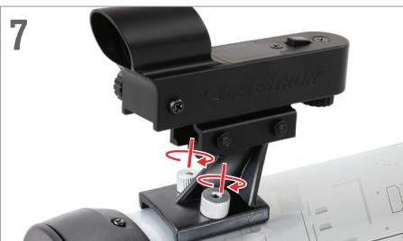
Place the finderscope over the threaded posts on the optical tube and secure the finderscope in place by tightening the knurled nuts from step 5.
