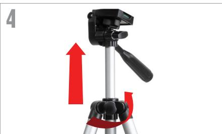
To extend the tripod's central column, loosen the collar on the mount by turning the locking knob counterclockwise, lift up the tripod head until it is at the desired height, and turn the locking knob clockwise to secure.
