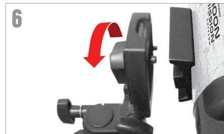
Match the 1/4"-20 threaded bolt in the mounting platform to the threaded 1/4"-20 hole on the bottom of the telescope tube and thread the two together by turning the upper mount knob clockwise. This should be tight, but be sure to not over-tighten.
