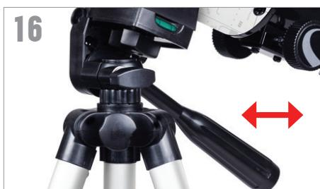
To move the scope right and left, hold a tripod leg with one hand while the other hand uses the panning handle to move the scope. The azimuth locking screw can be loosened or tightened to adjust the tension to your preference.
