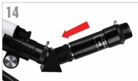
For additional magnification, you can use the included 3x Barlow lens. Place the Barlow lens between the diagonal and the eyepiece.
