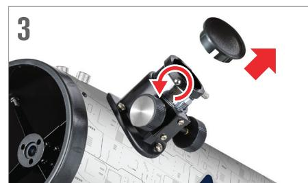
Next, remove the eyepiece cap and insert the 20mm eyepiece into the eyepiece tube. If necessary, back the thumbscrews out, so the threads are not impeding the insertion of the eyepiece.
