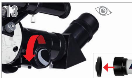
Remove the lens cap from the front of the telescope. To observe, look through the eyepiece as shown. Focus the image by turning the knobs below the focuser.
