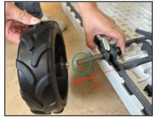
To assemble wheels push wheel axle pipe out and slide wheel onto axle pipe, until it clicks.
