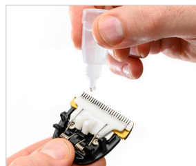
Adding lubricant onto the blades
