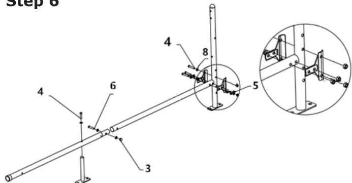
Connect the bars with the screw #6(1pc), washers #8(7pcs), nuts #5(4pcs), screws #4(5pcs) and the nut #3(1pc).
