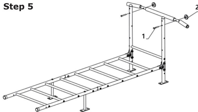
Install the pull-up bar to the SET with screws #1(2pcs) and knobs #2(2pcs).
