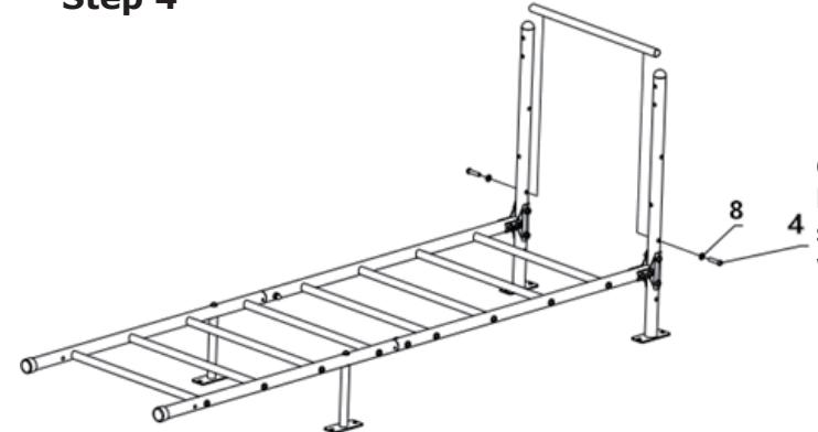
Connect the horizontal bar to the SET with screws #4(2pcs) and washers #8(2pcs).
