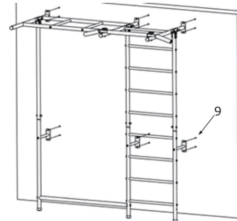
**Install the Set onto the Wall**
