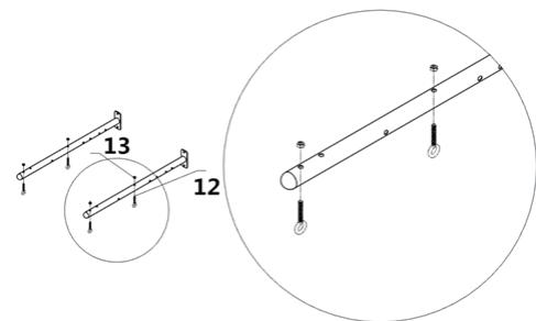
Install the screw #12(3pcs) and nuts #13(3pcs) on the bar, as picture above.
