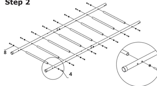
Install the horizontal bars to the vertical bars with screws #4(16pcs) and washers #8(16pcs).
