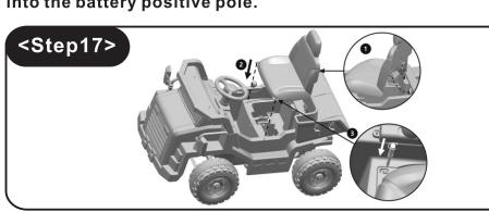
17. Place the seat into the body, then tighten by two screws with a screwdriver(not included).
