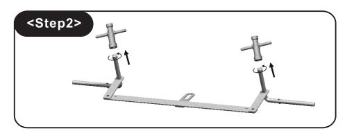
2. Loosen the two nuts by the tool provided.
