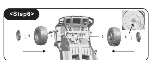
6.Insert the two washers first together with the two front wheels, tighten using a washer and a big cotter pin, then cover the wheel caps.
