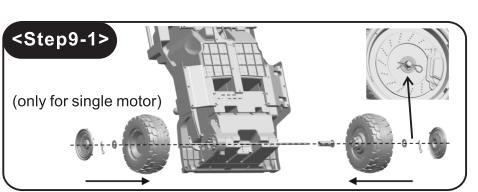
9-1(only for single motor)Insert the spacer from the right into the rear axle then insert the two rear wheels, tighten using a washer and a big cotter pin, cover the wheel caps at the end.
