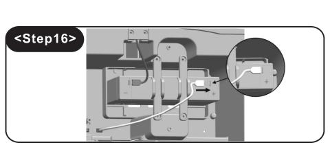
16. When the battery is installed, insert the red cable terminal into the battery positive pole.
