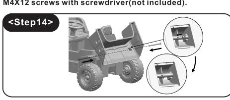
14.Insert the hopper axles, tighten using a small cotter pin as picture show.
