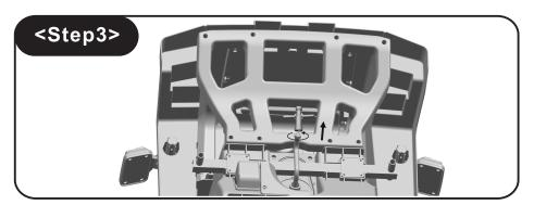
3.Loosen the nut under the body by the tool provided.
