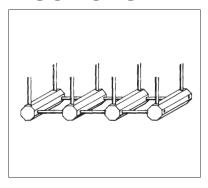
2. Add the vertical pins. If any wood pin seems loose, discard it and replace it with one of the spares.
