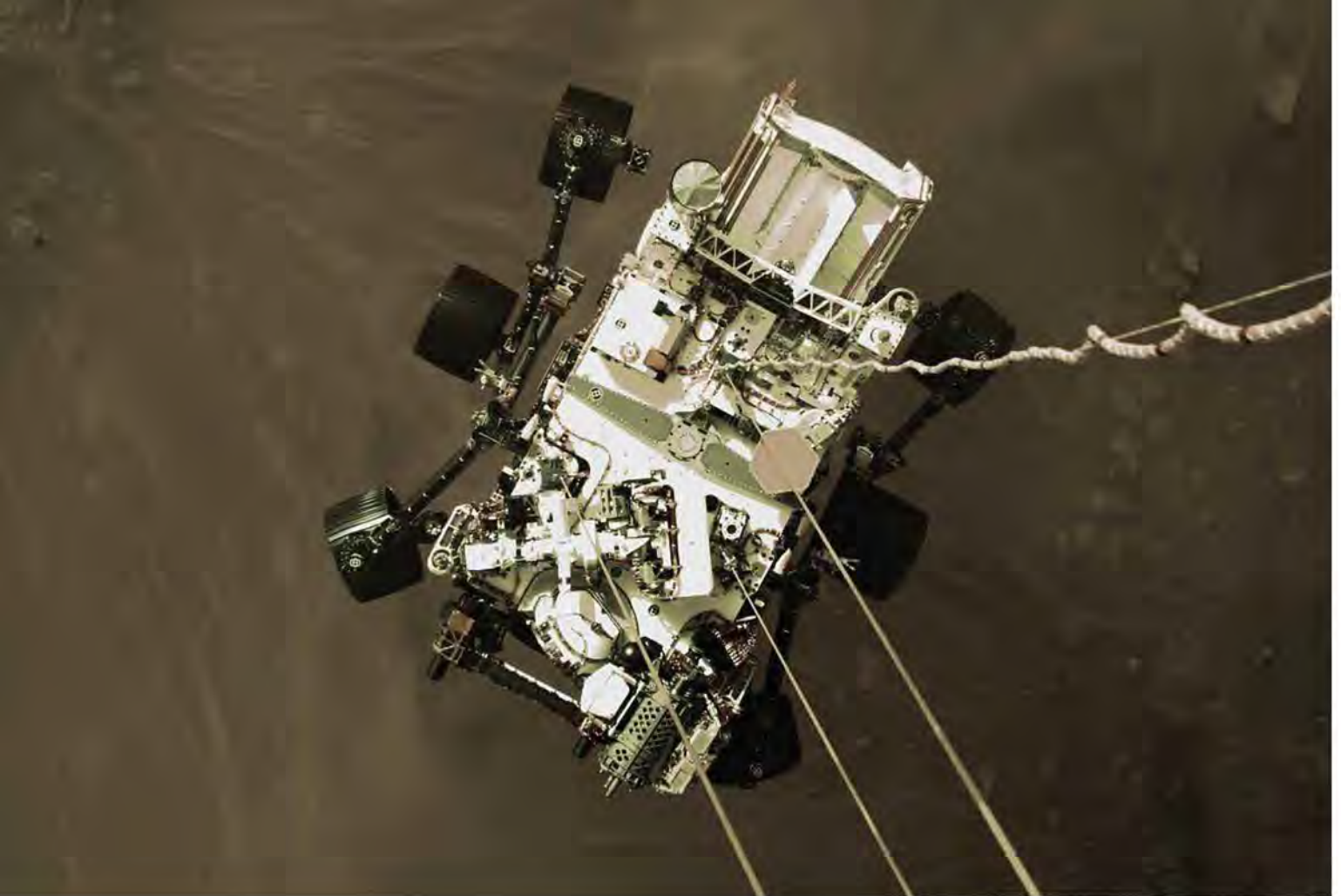
Perseverance Landing using Skycrane
