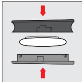
2. Twist to separate the top and bottom housings. Place AirTag between housings.
