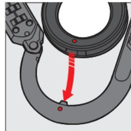
4. Place AirTag housing into carabiner; Make sure to align the dot on the housing to corresponding dot on the carabiner.
