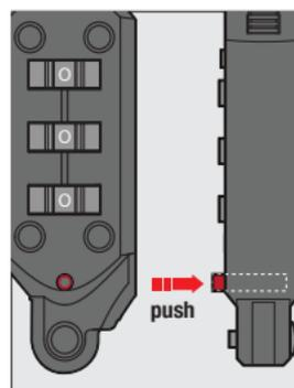
3. Finally, to set combination, press pin from backside to confirm the new combination.
