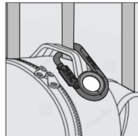
5. To lock carabiner, close latch and rotate digits to secure the lock.
