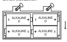
Remove screws and slide door to open
