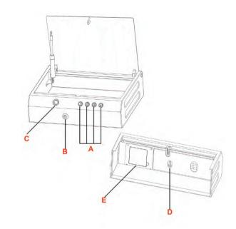
A: Digital Button (1 2 3 4 ) B: Keyhole C: Fingerprint Biometric Reader D: Setting/Resetting Button E: Battery Compartment
