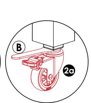
Tighten Castor completely
