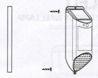
You can use the provided screws to fix the solar light in a suitable position. You can try other methods to install it according to the actual situation. But don't turn the wooden solar panel upside down, otherwise it will affect the effect of solar charging during the day.
