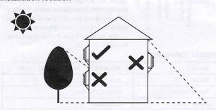
The solar light should be installed in a place with sufficient light to ensure that the solar panel can fully absorb the sunlight, thus extending the working hours of the solar light. The angle and the direction of the solar light should be adjusted to the best position, and the recommended best height is 2-3m.
