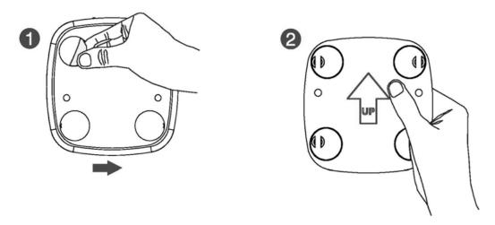
3. Align the holes on the back of the device with the pins on the bracket. Slide down to mount the device.
