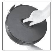
1. Place fingers into the finger inserts located on the top and bottom
