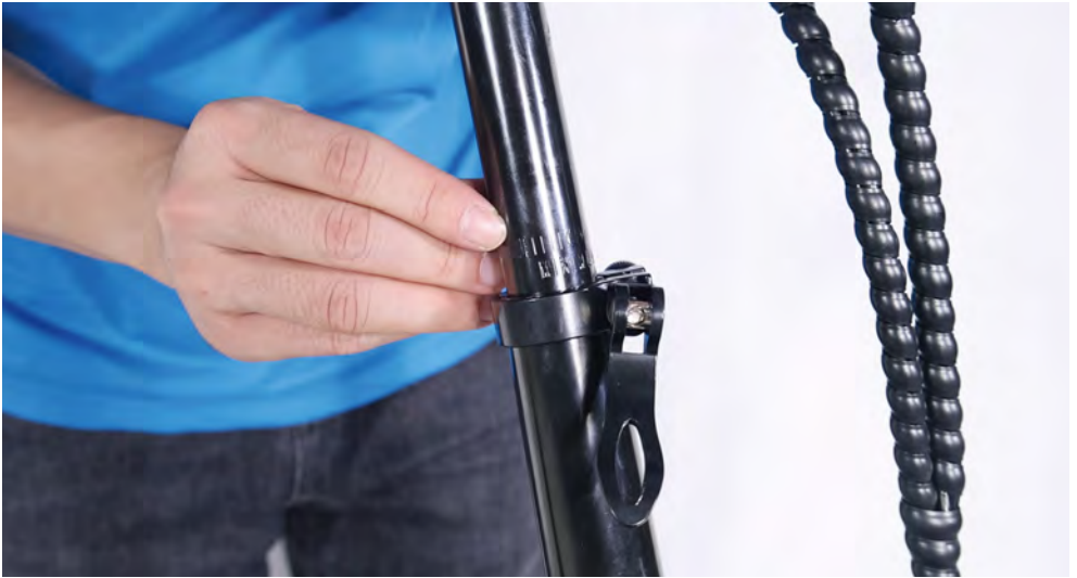
(4).Align the stem so the handlebar is perpendicular to the front wheel.
