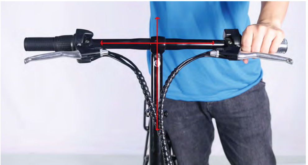
(5).Close the quick release lever to secure the handlebar.
