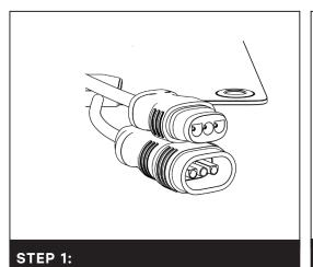
Align mat connector with Power Unit connector.
