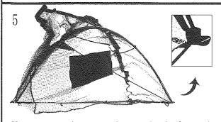
Now go to the opposite end of the pole and push the rest of the way into the sleeve with enough force to cause the pole to bow. Once you' ve inserted the pole all the way, insert the pin into the end of the pole.
