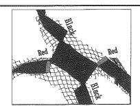
Lay net flat on the ground. Locate the center portion of the net that has the color coded Red & Black pole sleeve ends and position it in the center as you're laying out the net.
