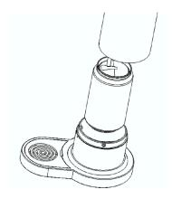
3. Replace the main body on the pedestal and turn clockwise. The parts are locked when the markings on the main body and pedestal are aligned.
