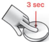
You can switch it off beforehand by pressing on the touchpad with your finger for 3 seconds.
