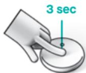
**ACTIVATE THE SETTINGS MODE.** Press down lightly on the touchpad with your finger for 3 seconds so that the LEDs light up. Please note that they shouldn't be flashing.
