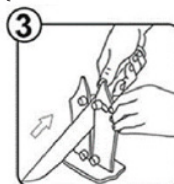
Hone for daily maintenance [metal is not removed].
