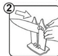
Hone for daily maintenance [metal is not removed].
