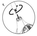
Insert the threaded end of the lower handle section (**D**) into the top of the VaBroom® Unit (**A**) and twist clockwise.
