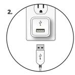
Insert the USB-A end of the charging cable into a USB power source.
