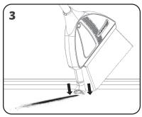
Point the nozzle opening at the start of your debris line. Gently push the nozzle against the floor to turn ON the vacuum suction.
