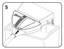
**TO EMPTY DEBRIS**, position the "Bombs Away Door" facing downward over the trash can (Vabroom® logo facing up)
