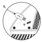
Insert the micro end of charging cable (**E**) into the charge port on the back of the VaBroom® Unit (**A**).
