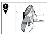
To remove mop pads, simply pull pads off the hook and loop material on the bottom of the machine.
