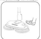
After inserting two AAA bateries, and powering up the main unit, you are now ready to turn on the unit with the buttons on the handle. Use the power button to activate the Dual Spin Mop. Use the Spray button to dispense liquid from the water tank.
