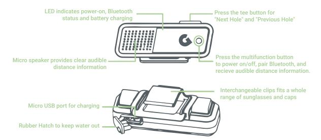
1. Turn GoGolf GPS on and pair to your smartphone by pressing and holding the side MULTIFUNCTION BUTTON (4) until the LED (2) on the side goes from red to an alternating red/green indicating it is ready to be paired. When paired, the LED (2) will be green. It should only be necessary to pair to a device one time.
